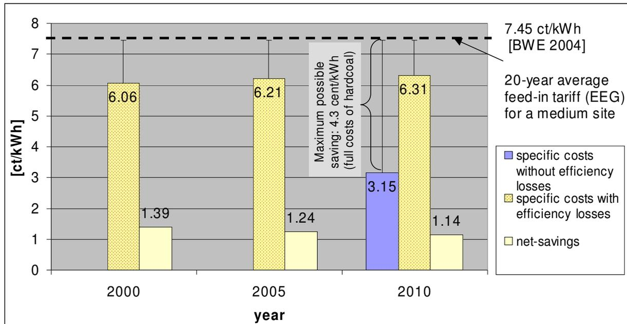
**Figure 25: Theoretical and actual specific costs of wind power feed-in**
