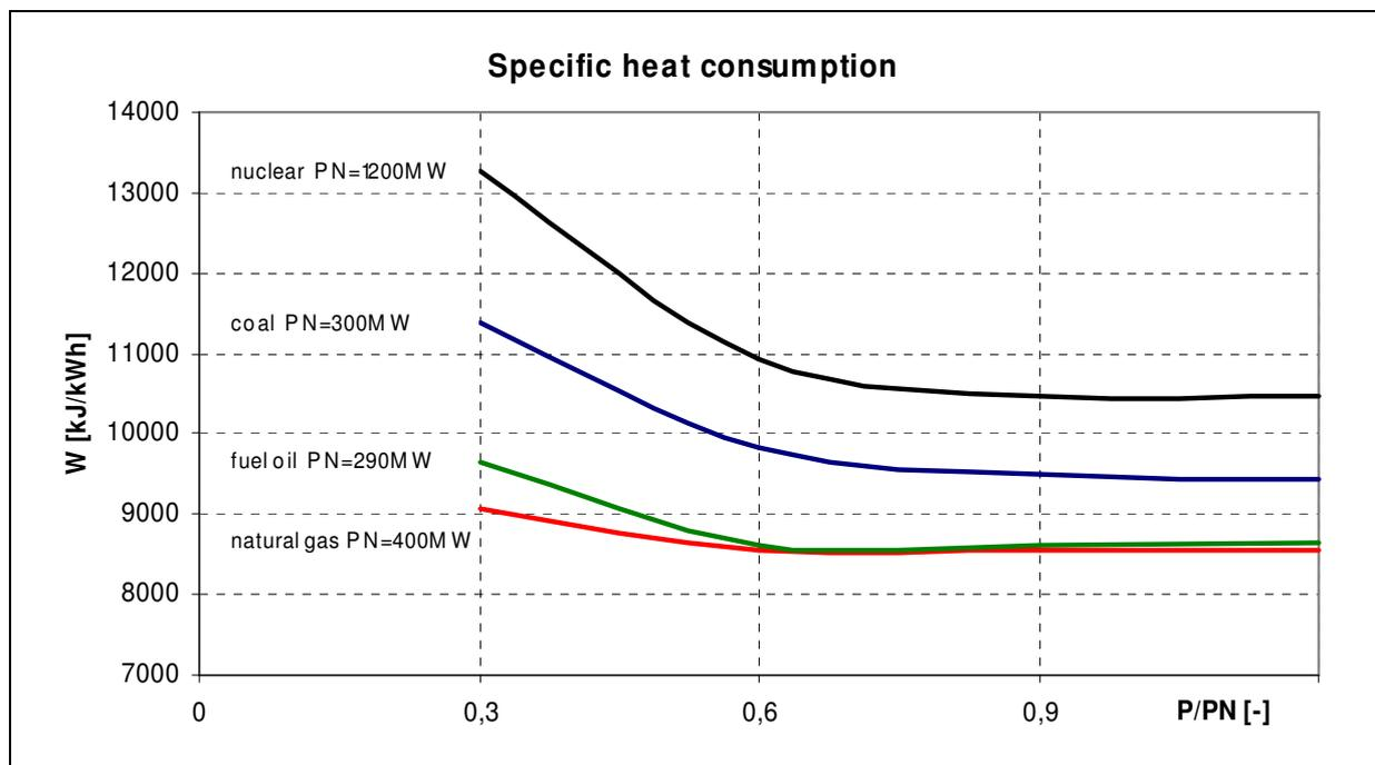
**Figure 22: Performance-related specific heat consumption of power plants (based on [Taud 1979])**
