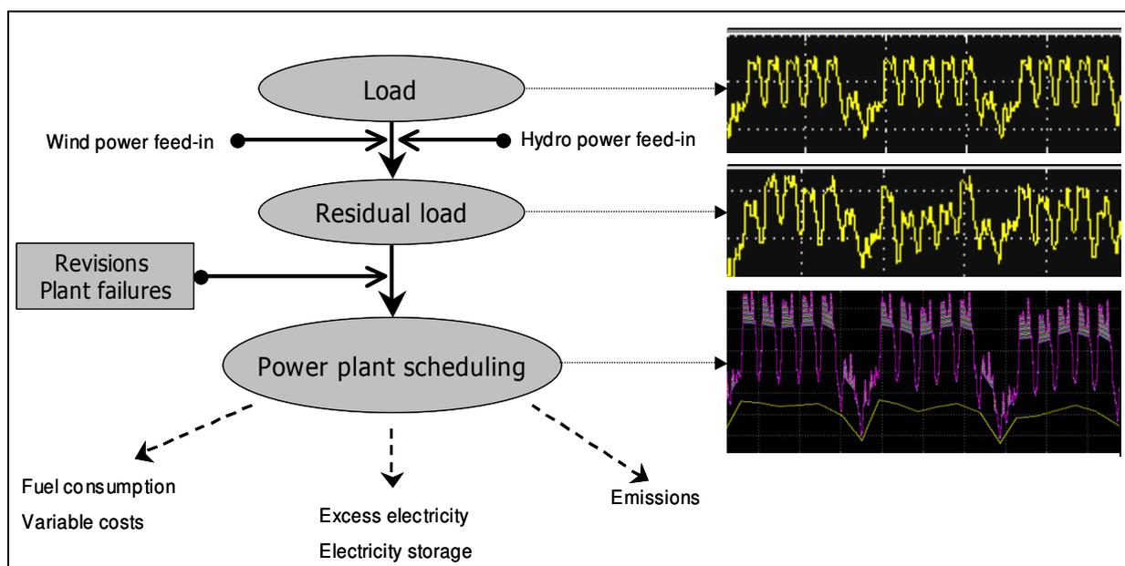
**Figure 17: Schematic overview of the AEOLIUS modelling approach**
